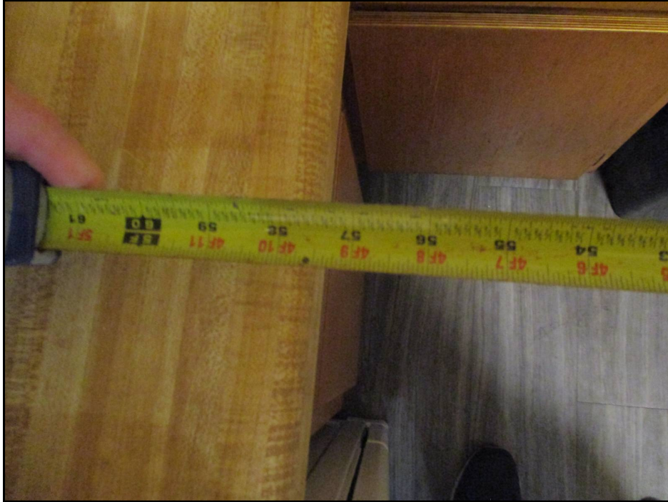
45: Non-Compliant Handicapped Dwelling Unit U-Shaped Kitchen Clear Floor Space (Critical Repair)
